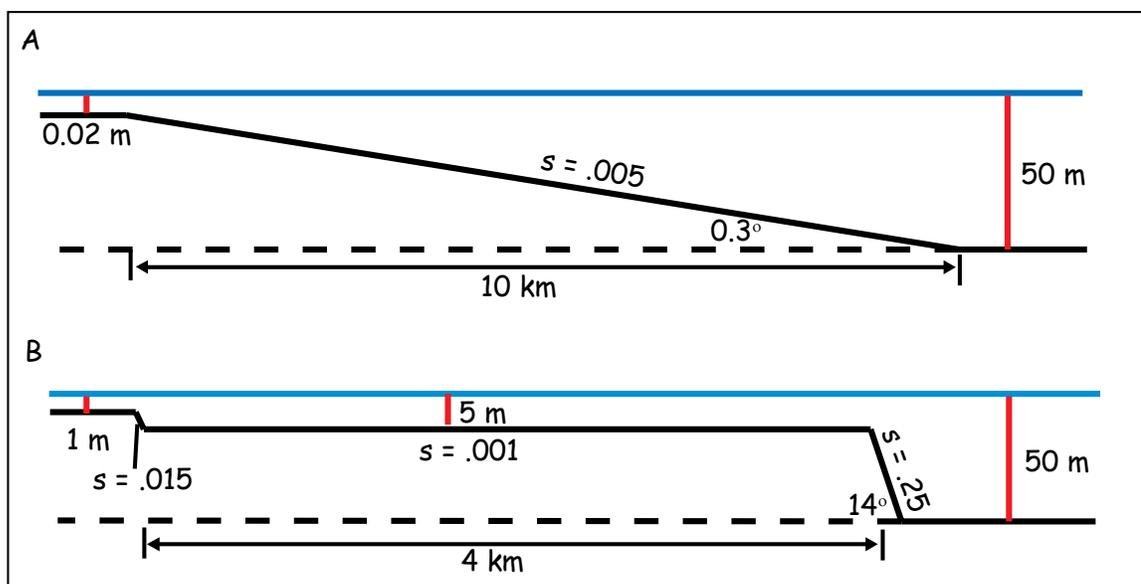
Figure 6: Bathymetric configurations for the ramp (A) and platform (B) situations modeled with the wave model. The platform bathymetry (B) consists of 3 different slopes used to determine the breaking criteria for the waves.
