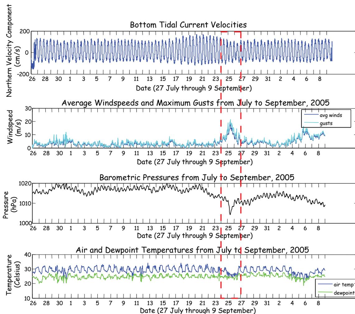
Figure 9: Comparison of the northern component of the tidal forcing at the bottom of a tidal delta (top) with atmospheric effects (NOAA buoy, bottom three plots) in late summer, 2005. The measurements were obtained by an ADCP located at ADCP1 in Figure 1. Although the presence of the storm (Hurricane Katrina, red dashed box) is obvious in the atmospheric data, it does not appear as obvious in the tidal measurements. Note that the average tidal velocities exceed 1 m/s, daily.
